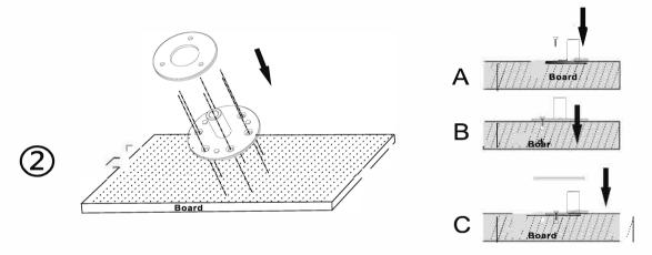
Step 3. Place the safe down over top of the anchor and fasten with the Allen bolt.
