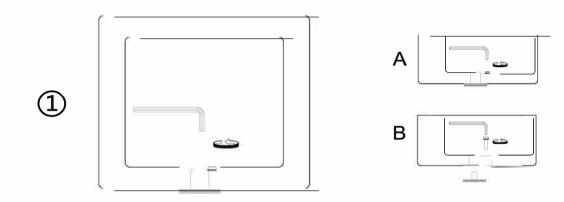
Step 2. Fasten the anchoring device to the floor using the included screws.
