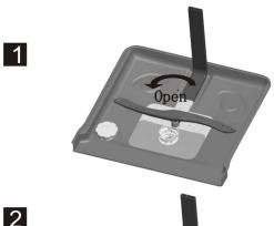
Step 1: Turn the filter in anti-clockwise direction,
